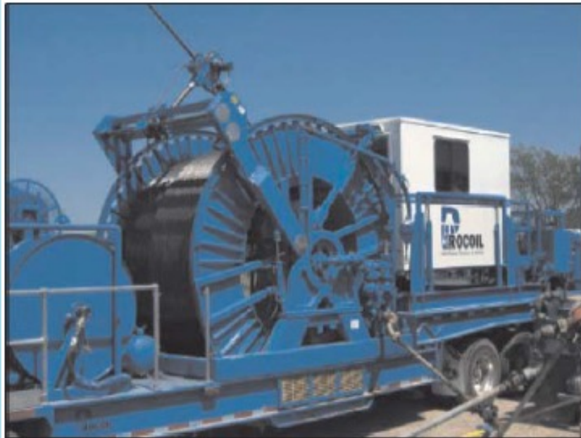
Figure 7 CT surface operation unit
